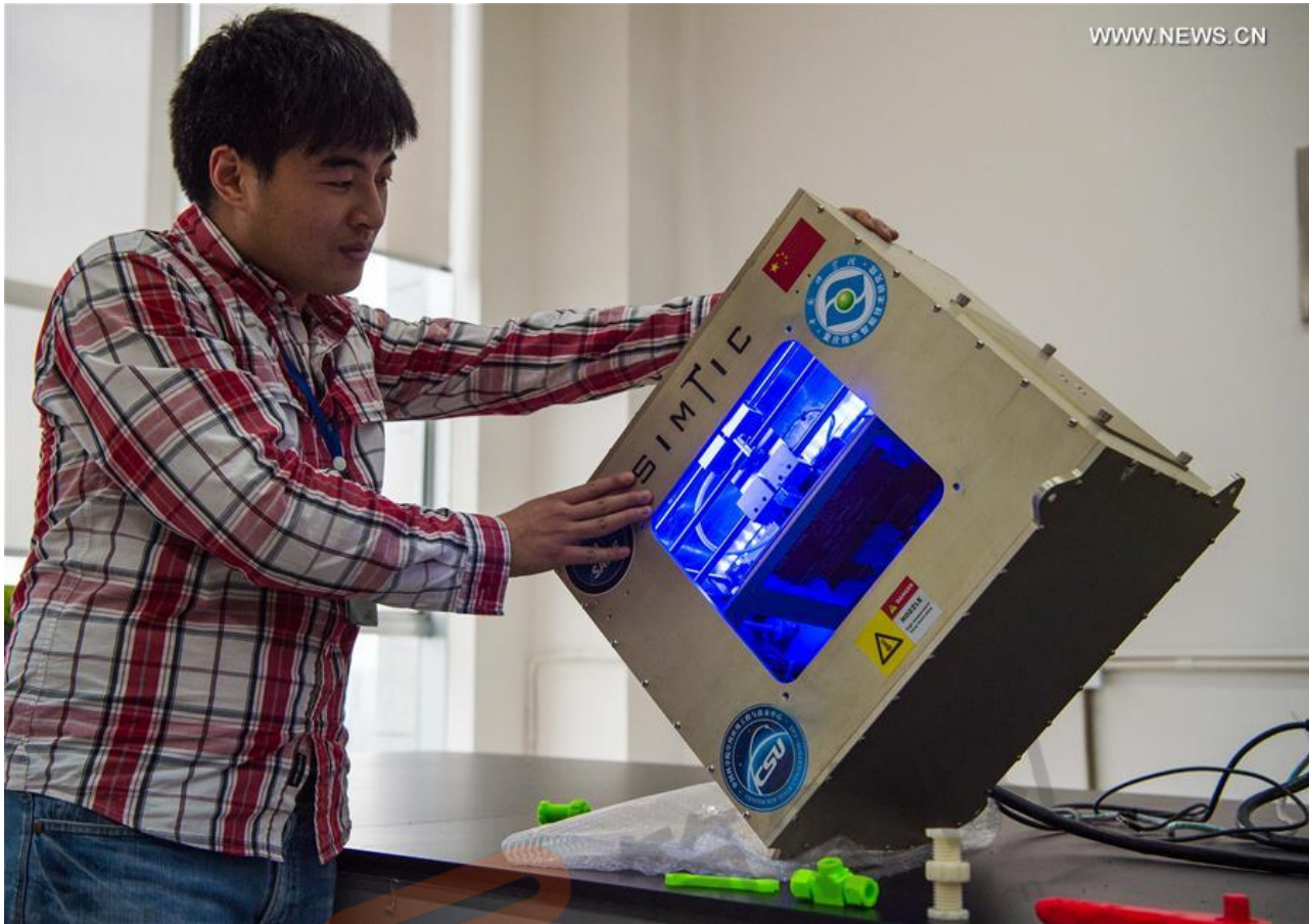
A micro-g 3D printer works in a tilting status at a research center in southwest China's Chongqing Municipality, April 19, 2016. The Research Center for Additive Manufacturing (3D Printing) Technology of Chongqing Institute of Green and Intelligent Technology announced on Tuesday that the first micro-g 3D printer was successfully developed. (Xinhua/Liu Chan)
