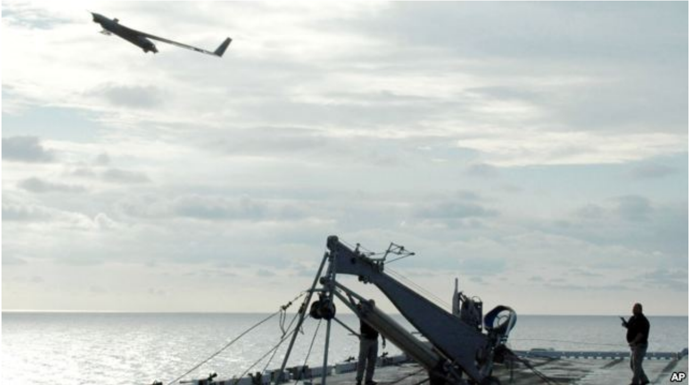
A Scan Eagle unmanned aerial vehicle launches from the flight deck of an amphibious assault ship. (File)
